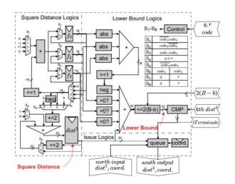
BDU Verilog Implemented by Us: <a href="https://github.com/EECS-573-KNN-Accelerator/eecs573project/blob/main/verilog/BDU.sv">https://github.com/EECS-573-KNN-Accelerator/eecs573project/blob/main/verilog/BDU.sv</a> Run the BDU test here: <a href="https://github.com/EECS-573-KNN-Accelerator/eecs573project/blob/main/test/BDU">https://github.com/EECS-573-KNN-Accelerator/eecs573project/blob/main/test/BDU</a> test.sv
